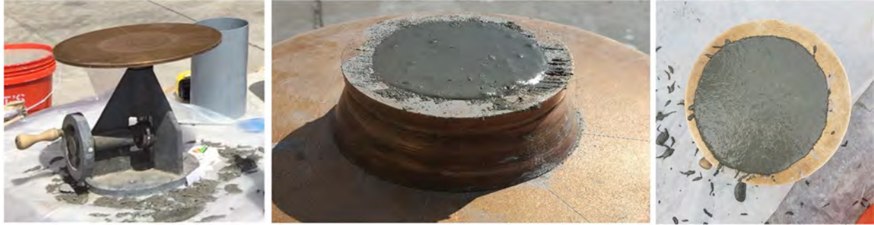
Figure 2.9 UHPC flow testing.
