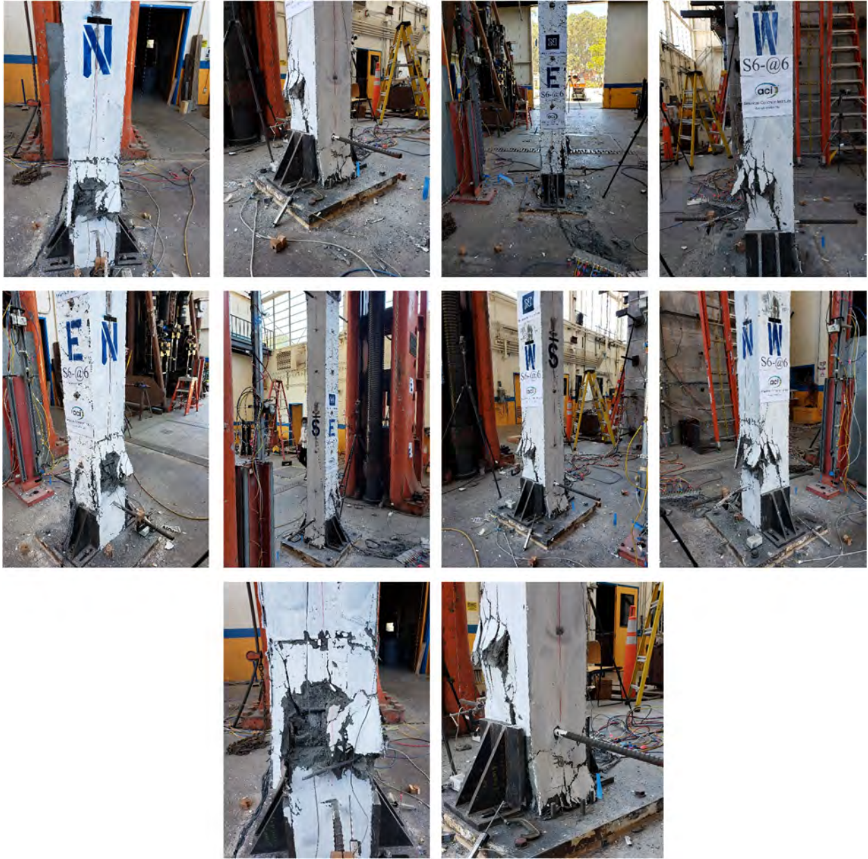
Figure C.6 Final damage state of column S12-H6.
