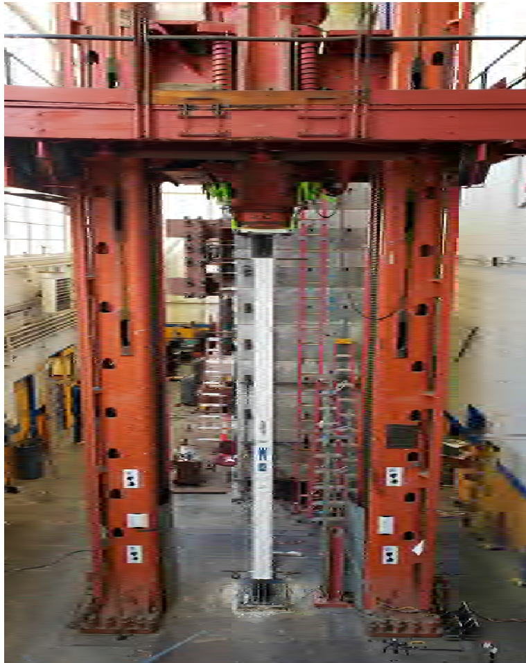
Figure B.18 Final test setup of the column.
