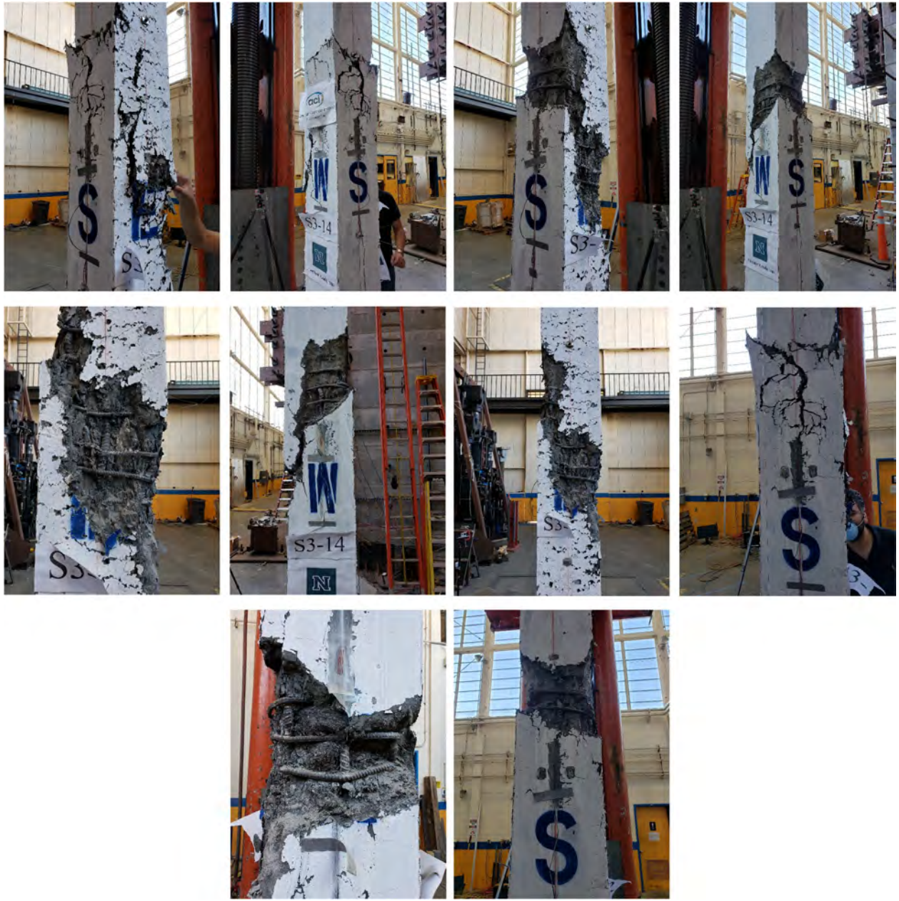
Figure C.3 Final damage state of column S14.
