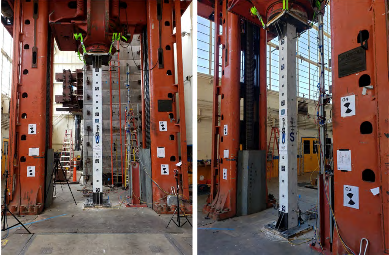
Figure 2.12 Typical full-scale UHPC column test setup at PEER Laboratory.
