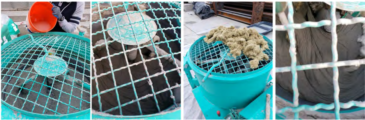
Figure B.5 UHPC while being mixed in the high shear mixer.
