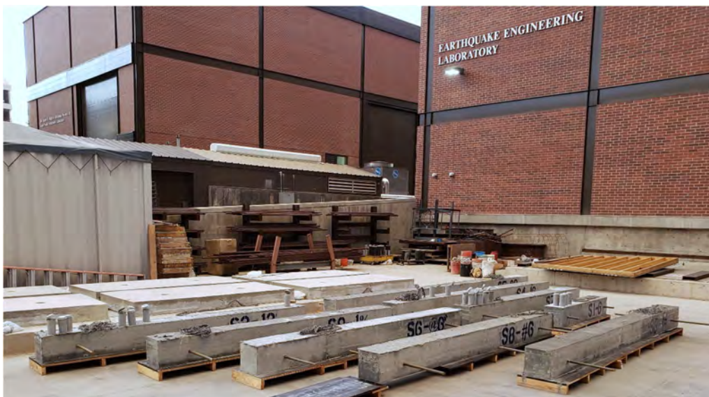
Figure B.9 UHPC columns after construction and ready to be transported
