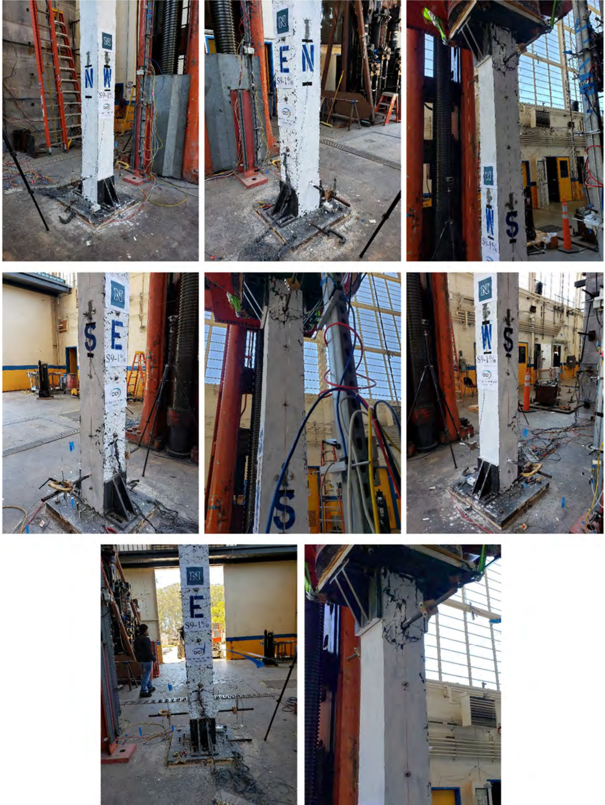
Figure C.9 Final damage state of column S12-F1.
