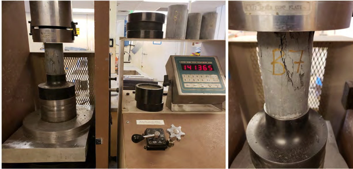
Figure 2.10 UHPC compression test setup and typical mode of failure.
