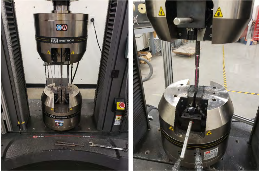
Figure 2.11 Direct tension test setup for rebar samples.
