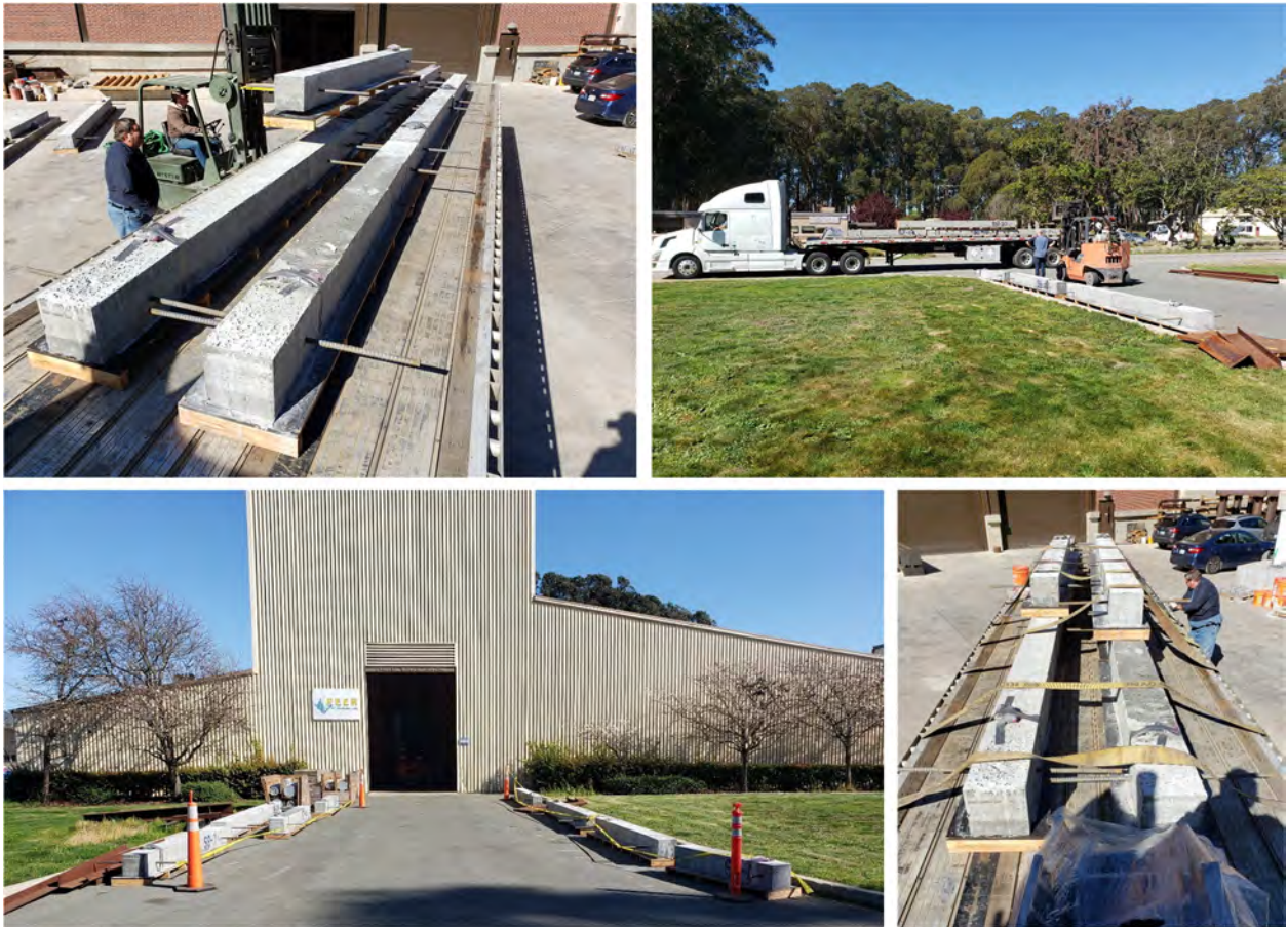
Figure 2.7 UHPC columns transportation from UNR to PEER Laboratory.
