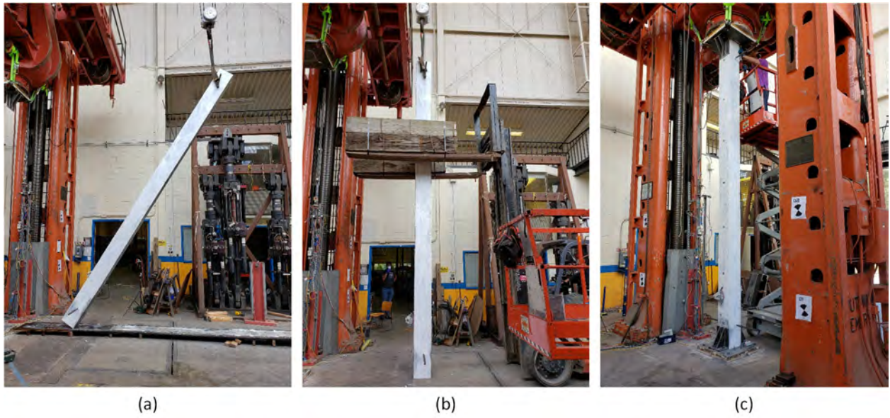
Figure B.17 (a) holding the column in a vertical direction using the crane, (b) driving the column underneath the machine using a forklift, (c) attaching the two end fixtures and tightening them.
