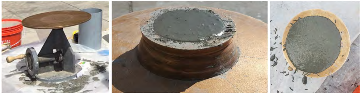
Figure B.6 UHPC flow testing.
