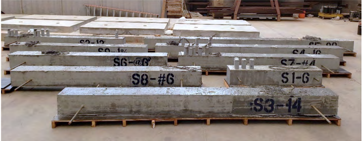
Figure 2.6 UHPC columns after construction and ready to be transported.
