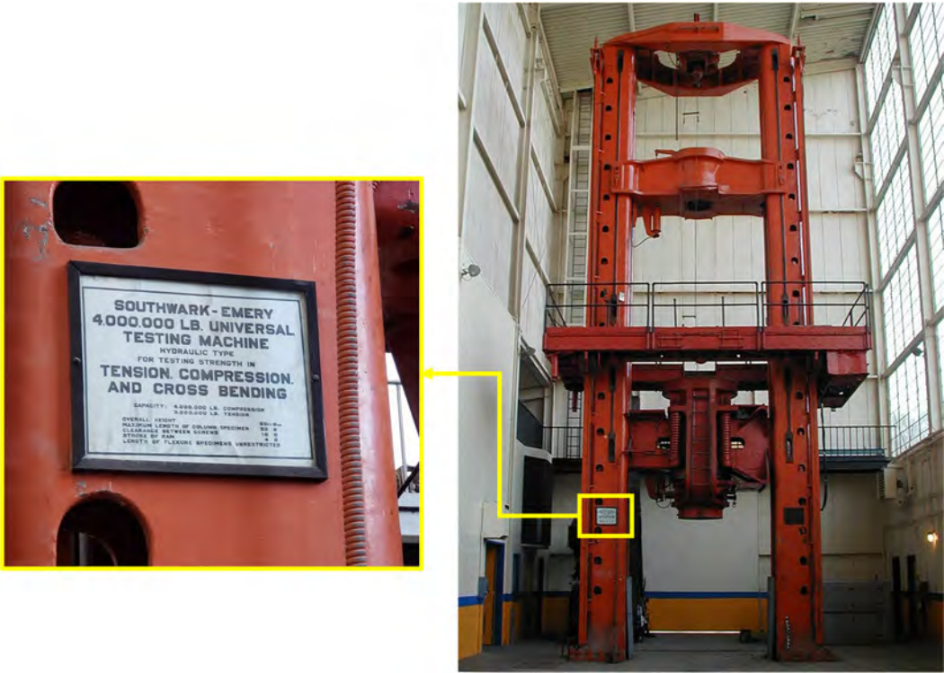
Figure 2.13 The 4,000 kip [17,793 kN] loading frame at UC Berkeley PEER Laboratory.
