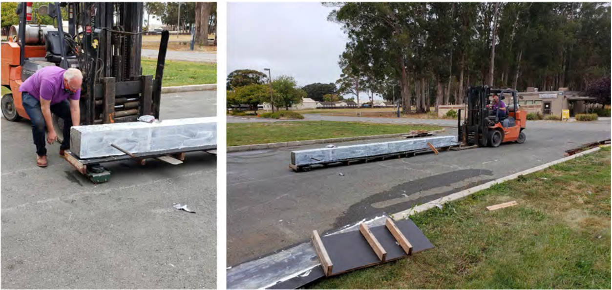
Figure B.16 Putting a roller underneath the column and driving it inside the lab.
